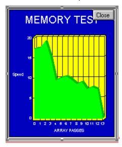
The high speed on the left end of the chart (17MB per second in this case) represents how fast your CPU can perform a series of read/write operations inside the 8KB primary cache. The low speed on the right end of the chart (6MB per second) indicates the speed of the main RAM on the motherboard. Installing 256KB of secondary cache changes the figure to look like this:
